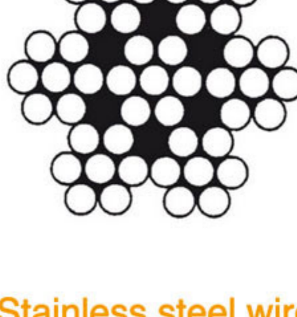
Stainless steel wire rope medium soft 7x7 8379
