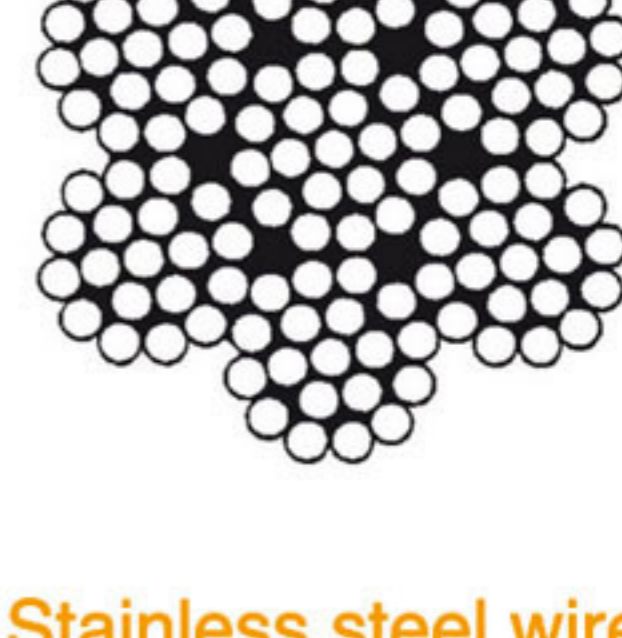
Stainless steel wire rope flexible 7x19 8382
