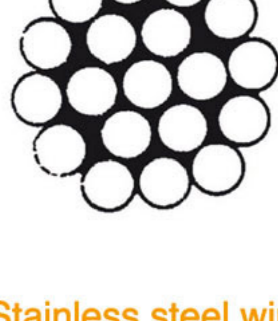
Stainless steel wire rope hard/ rigid 1x19 815068
